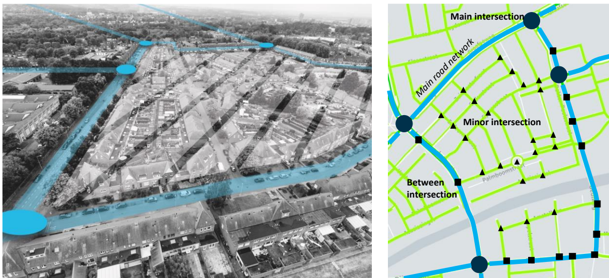
Figure 3: an example of how the VIA Clustered Road Network (VCRN) algorithm fully automated divides the complete nationally road network into clusters of intersections and road sections to combine different data types into a mutually comparable reporting level
